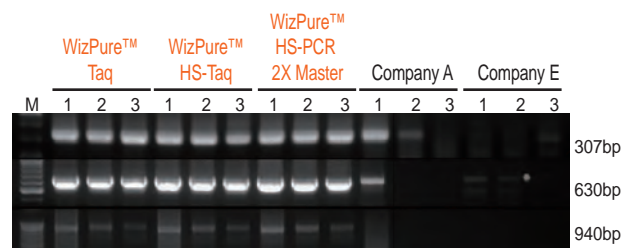
Fig 2. Comparison of PCR performance with Wizbiosolutions and competitor's PCR Master mix kit using different PCR product size. Lane M (100bp ladder), Lane 1~3 : 10-fold dilution of template DNA, PCR : 35 cycles.
