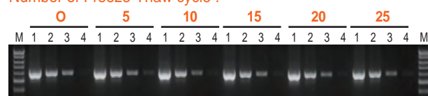
Fig 3. Stability of WizPure™ HS-PCR 2X Master (UDG) through multiple freeze-thaw events. Freeze-thaw events were performed by allowing PCR 2X Master (UDG) to thaw from -20°C to room temperature. A 630bp fragment was amplified using the PCR 2X Master (UDG) after 25 freeze-thaw cycles. Lane M (100bp ladder), Lane 1~4 : 10-fold dilution of template DNA PCR : 35 cycles.
