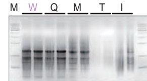
Fig 2. Total RNA was purified from 100 mg leaf samples of Brassica rapa var. glabra using the WizPrep™ Plant RNA Mini Kit and competitors. 7 µl of the eluate (elution volume 50 µl) were analyzed on a 1.5% agarose gel. M: 1kb DNA ladder, W: Wizbio, Q: Competitor Q, M: Competitor M, T: Competitor T, I: Competitor I.
